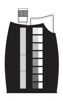
The Octa-Slide 2 Viewer should be held so non-direct light enters through the back of the Viewer. Slide the Octa-Slide 2 Bar into the Viewer. Insert the reacted sample into the top of the Viewer. Match the color of the reaction to the color standards.
