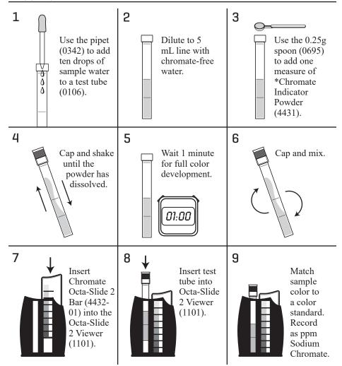
If the color of the test sample is less than the color of the lowest standard, repeat the test using a sample of the water without dilution and divide the value of the standards by ten. If the color of the test sample in the original test is deeper than the highest value, the test is run again with a more dilute sample. See Dilution Factor Table.
