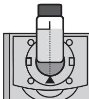
6. Remove tube from colorimeter. Add one DPD #1 IG Tablet [6903A]. Cap tube and shake for 10 seconds. Invert slowly 5 times. Solution will turn pink if free chlorine is present.
