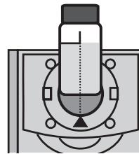
11. Subtract free chlorine reading from total chlorine reading to obtain concentration of combined chlorine.
