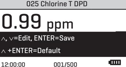
10. Press or to adjust the value shown to the concentration of the prepared standard, 1.00 in this example.
