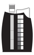
The Octa-Slide 2 Viewer should be held so non-direct light enters through the back of the Viewer. Slide the Octa-Slide 2 Bar into the Viewer. Insert the reacted sample into the top of the Viewer. Match the color of the reaction to the color standards.
