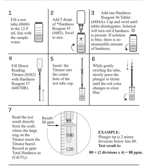
**NOTE:** If the plunger reaches the bottom line on the scale (200 ppm) before the endpoint color change occurs, refill the Titrator and continue the titration. When recording the test result, be sure to include the value of the original amount of reagent dispensed (200 ppm).
