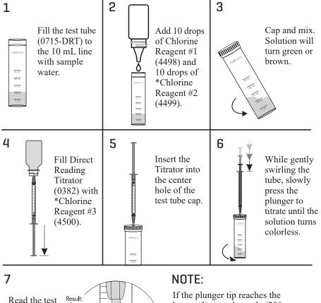
Read the test result. Result directly from the scale where the large ring on the Titrator meets the Titrator barrel. Record as ppm Chlorine.
