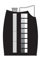
The Octa-Slide 2 Viewer should be held so non-direct light enters through the back of the Viewer. Slide the Octa-Slide 2 Bar into the Viewer. Insert the reacted sample into the top of the Viewer. Match the color of the reaction to the color standards.
