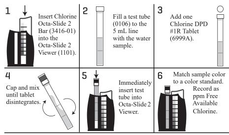
NOTE: Recommended Minimum Free Available Chlorine level in spa water and hot tubs is 3.0 - 5.0 ppm, and in pools 1.0 - 3.0 ppm.
