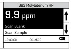
NOTE: The meter will remember the last scanned blank reading. It is not necessary to scan a blank each time the test is performed. To use the previous blank reading, instead of scanning a new one, scroll to Scan Sample and proceed. For the most accurate results, the meter should be blanked before each test and the same tube should be used for the blank and the reacted sample.
