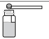
Cap and invert to mix until the powder dissolves. Solution will turn yellow if molybdenum is present.
