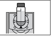
8. Remove tube from colorimeter. Use the 0.05 g spoon (0696) to add 0.05 g of \*Molybdenum Indicator Powder (6486).
