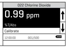
10. Press enter to select **Calibrate**. A reverse font (light background with dark characters) will appear to indicate that the reading can be adjusted.
