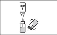
NOTE: For wastewater samples, <u>Standard Methods for the Examination of Water and</u> <u>Wastewater</u> recommends waiting 2 minutes for full color development when testing total chlorine. 10. Insert tube into chamber, close lid and select **Scan Sample**. Record result as Total Chlorine (Monochloramine, Dichloramine, and Nitrogen Trichloride) present in the water sample.
